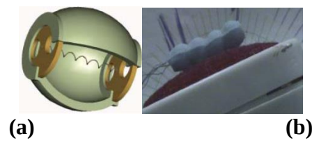
Fig. 19 (a) Earthworm module, (b) The artificial earthworm [18].
